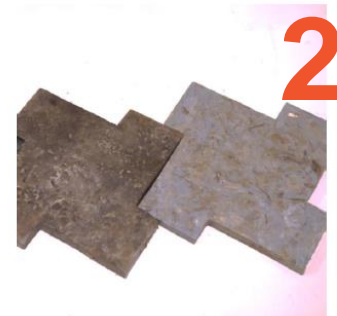
Biocomposites using Pinyapulp and Pineapple Leaf Fiber (PALF) Waste via Compression Molding by Manila Automat
