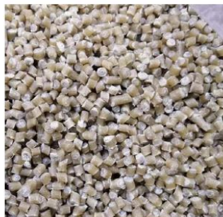
Bio-composite pellets using Pineapple Leaf Fiber (PALF) Waste via Twin Screw Extruder by DOST-ITDI
